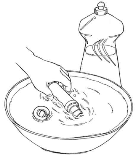
Sawirka 3 Nadiifi aalada caawisa caaga daawada lagu dhuuqo, qalabka dambe ee aalada iyo maaskarada hal mar asbuucii adoo adeegsanaayo midkood gacantaada ama saqafka mashiinka weelasha lagu dhaqo.
